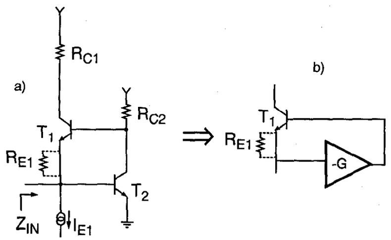
Figure 2: Feedback loop used to reduce the input impedance component dependent on the signal. The transistor  $T_2$  and its collector resistor  $R_{C2}$  amplify the base-emitter voltage of the input transistor  $T_1$ . Hence,  $T_1$  input impedance is reduced by the loop gain  $G$ . The resistor,  $R_{E1}$  ( $\sim 100 \Omega$ ) in series with the emitter is necessary to stabilize the loop. The resulting input impedance is:  $Z_{in} = (1/g_{m1} + R_{E1})/G$ .
