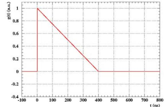
$$i(t) = i_0 \left( 1 - \frac{t}{t_d} \right) = \frac{en_e V}{d} \left( 1 - \frac{t}{t_d} \right)$$
