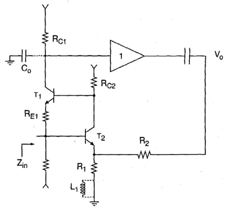
Figure 3: Simplified circuit diagram of the line terminating preamplifier. The external feedback loop increases the input impedance of the  $T_1 - T_2$  inner loop to the value:  $Z_{in} = (1/g_{m1} + R_{E1})/G + R_{C1} \times R_1 / (R_1 + R_2)$ . The addition of the inductor  $L_1$  in series with  $R_1$  achieves a pole-zero cancellation of the pole  $R_{C1} \times C_0$ , thus extending the bandwidth.
