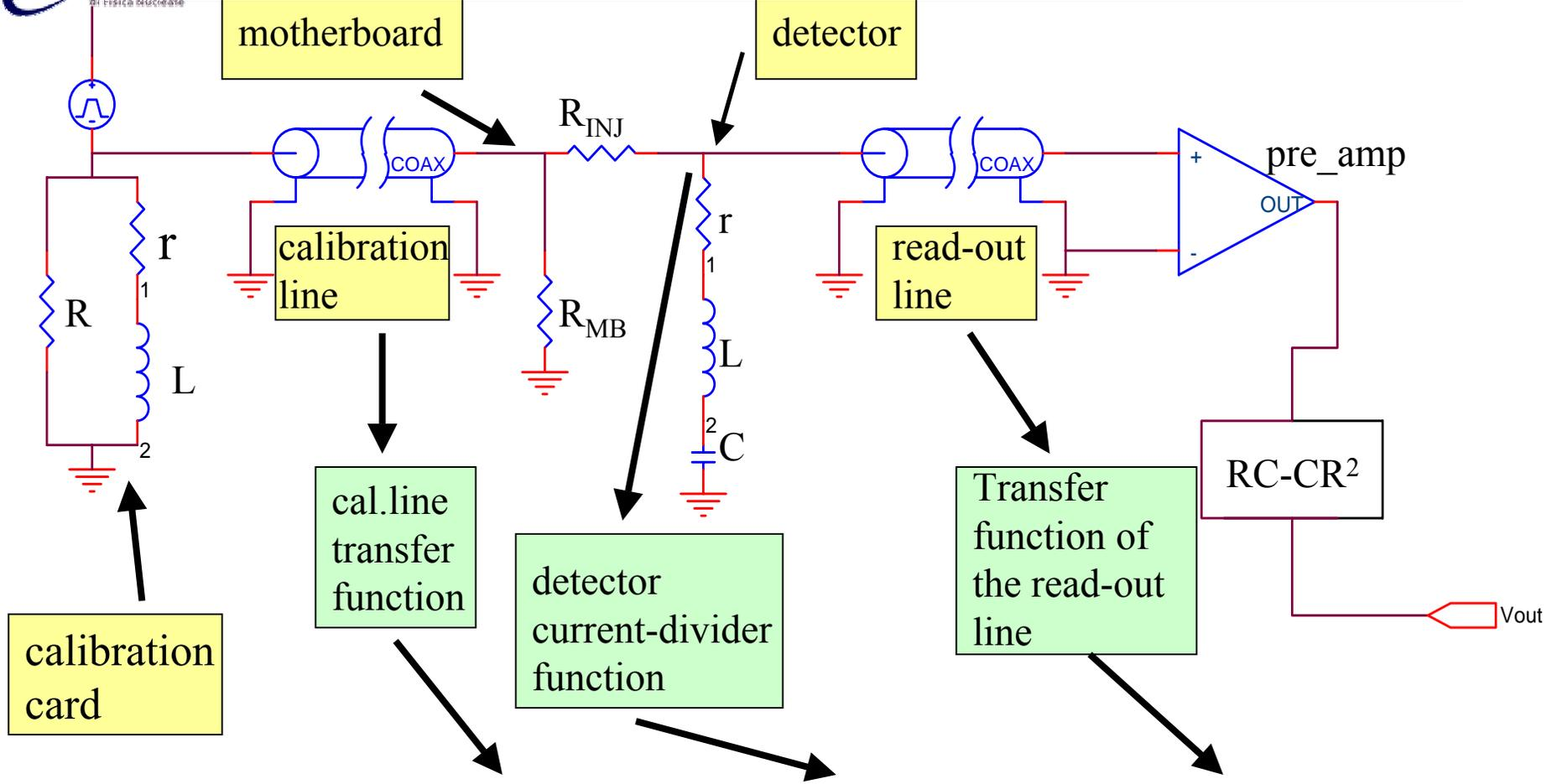
$$g^{cal}(s) \propto \frac{f_{step} + sT_{cal}}{s(1 + sT_{cal})} \cdot H_{cal}(s) \cdot \frac{1 + s^2LC + srC}{1 + s^2LC + s(r + Z_{ro}(s))C} \cdot H_{ro}(s) \cdot \frac{sT_{sh}}{(1 + sT_{sh})^3}$$
