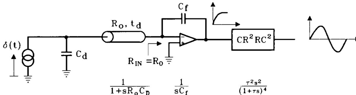
Fig. 2. Analog signal processing chain for the signal calculation. The preamplifier input impedance is tuned to terminate the transmission line ( $R_{in} = R_o$ ). The preamplifier input capacitance is disregarded. An additional signal attenuation is due to conductor losses in the transmission line (see appendix A). A  $RC^2-RC^2$  filter, giving a zero-area bipolar response to avoid baseline shifts at high rates is assumed.
